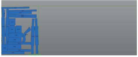
Marker name: RED LAYPLAN-150 Utilization: 67,39% Length: 1m 16.99cm Model/Size/Oty: RED LAYPLAN 12/1 Width: 150,01cm Unplaced/Placed: 0/22 The totally amount of fabric used for pieces consisting of Wine Red Duchess Satin is 1.2 Metres. Within this lay plan, there is a utilization of 67%. This suggests that there is a 33% fabric wastage from this fabric. This wastage can be used as spare material or may be used to create accessories.
