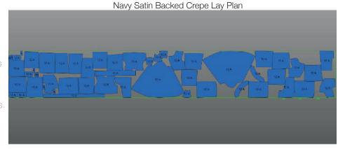
Marker name: BLUE LAYPLAN-112 Utilization: 75.72% Length: 7m 96.70cm Model/Size/Oty : BLUE LAYPLAN 12/1 Width: 111.99cm Unplaced/Placed: 0/52
